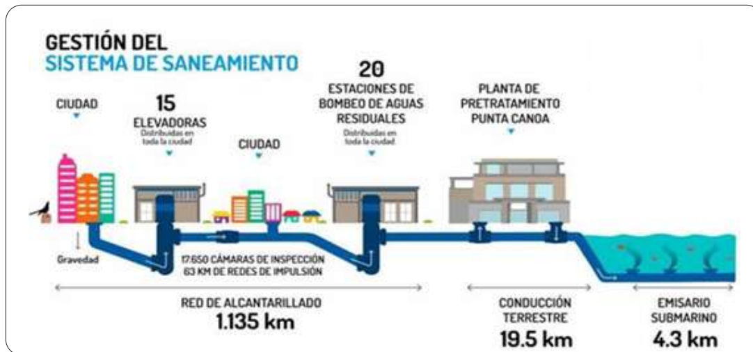
Illustration 82 Diagram of the wastewater treatment system in Cartagena.
